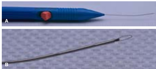
Figure 25. (A) The Yoshi Loop (Dental Cadre), a stainless steel micro-lasso that extends from the end of a stainless steel cannula attached to a handle with a retraction button for tightening the loop around a file segment; (B) Magnified view of the cannula and stainless steel micro-lasso.
