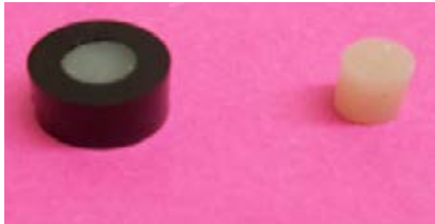
Figure 2: Composite specimens packed into Teflon moulds.
